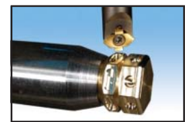
Drilling and milling a groove
