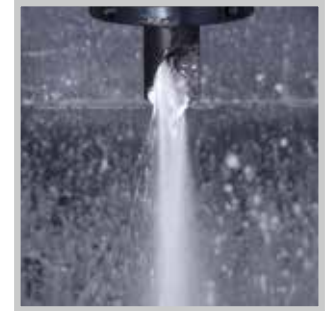
• High pressure coolant can be supplied through center directly to tip of center drill insert.
